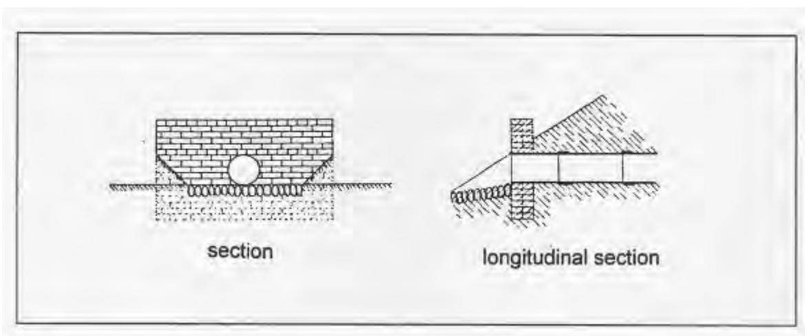
Figure 3.16. End elevation and longitudinal section of a pipe culvert under an embankment (Johnson 1899: 273, Fig. 8).
