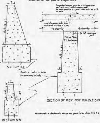
SECTION OF PIER FOR DOUBLE SPAN
