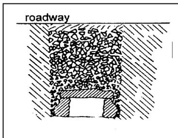
Figure 1.1. Drawing of stone culvert
