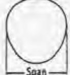
Span<br>25-30 ft                                                              | Grade separations, culverts, storm sewers, tunnels.                                                                                                            |
