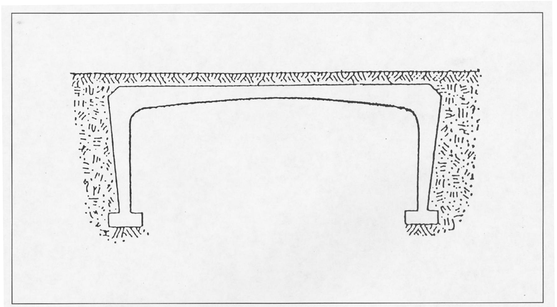
Figure 3.12 Rigid frame structure (Source: Spero 1995: 171).
