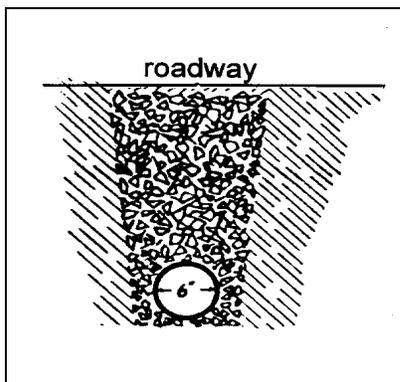
Figure 1.2. Drawing of a culvert
